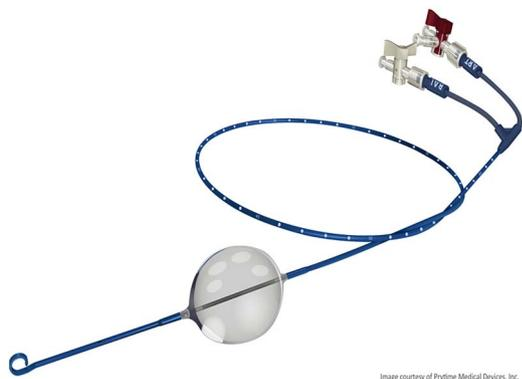
**Figure 1** ER-REBOA catheter. Design features include low-profile 7 French sheath designed for percutaneous insertion, stiff catheter that does not require the Seldinger technique or a guide-wire for insertion, curled catheter tip to minimize aortic injury and malposition, centimeter markings on the catheter to aid in blind positioning, and a proximal aortic blood pressure transducer.
